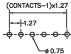
Recommended P.C.Board Layout
