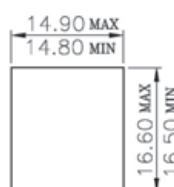
Front Panel Jack Only Clearance W/O Latch Feature
