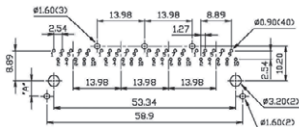
Recommended P.C.Board Layout
